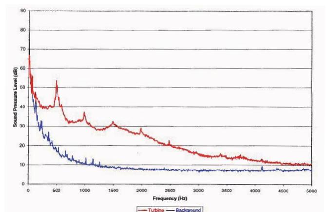
Narrow-band spectrum with tonalities of a wind turbine during acoustic measurement in the free field
