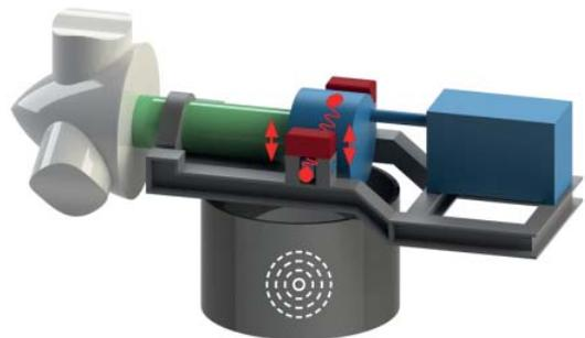
Preventing propagation and emission with absorbers at the gearbox
