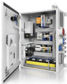
Feeder box for lighting systems For 48V DC feed-in to our Fieldpower LED tower lighting. In the event of power loss, continued operation is ensured for 60 minutes.
