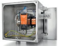
Anemometer junction box For connecting the power supply and signal transmission lines to the anemometer. An additional built-in surge protection module protects the downstream of electrical components in the event of a lightning strike.
