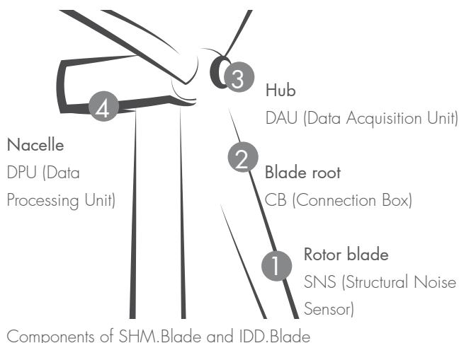
For IDD.Bla de and SHM.Bla de Basic, one sensor per rotor blade is sufficient. In case of higher requirements in terms of precision and redundancy, SHM.Bla de Standard can be used with two sensors on each rotor blade.
